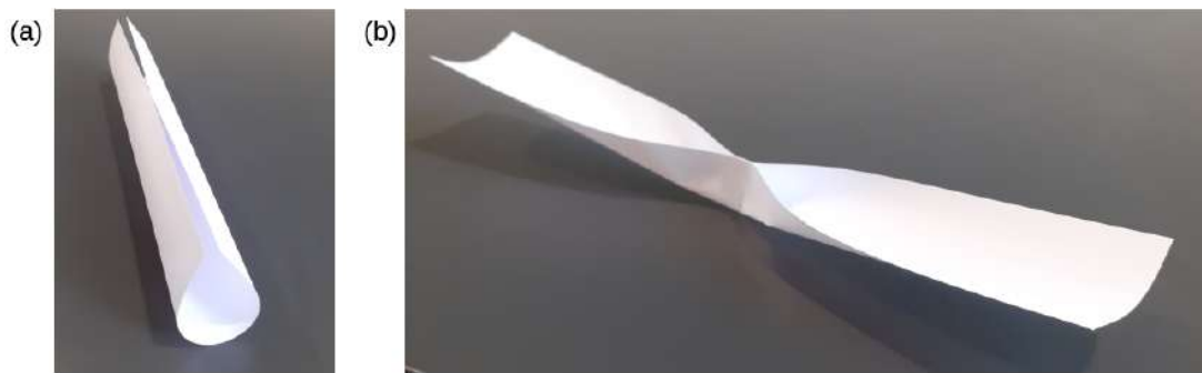
Figure 1. (a) Photograph of a rectangular paper strip ( L = 29.7 cm, W = 15 cm, t = 0.1 mm) with mid-length points at contact and maintained by an adhesive strip. (b) Photograph for a strip with a smaller width ( L = 29.7 cm, W = 5 cm, t = 0.1 mm).
